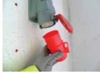
2. Insert the device fully into the socket ensuring correct alignment.
