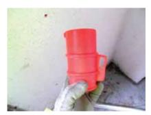
1. The lockout device has no internal parts and comprises of one single moulded part.
